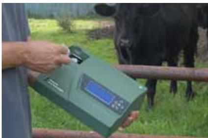
**This instrument is being tested for detecting BVDV in cattle.**
